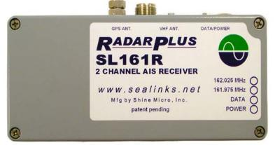
The **RadarPlus SL161R** is an easy to install, stand alone marine receiver that monitors the channels assigned to the **Automatic Identification System**, or **AIS**. **AIS** reports:
